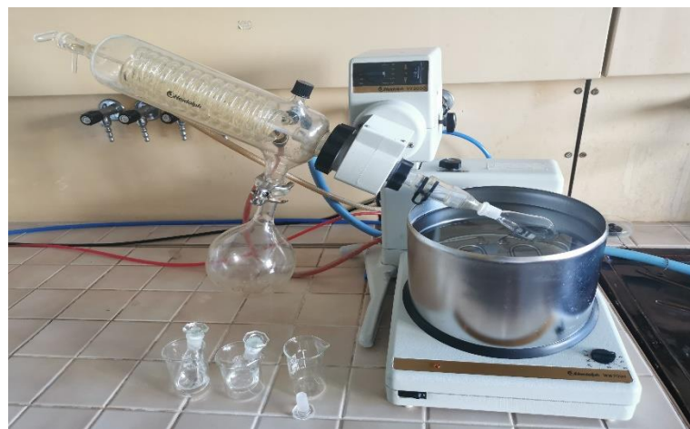
Fig. 5 Evaporation of collected ethyl acetate layers by rotary vacuum evaporator
