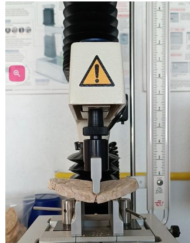
HDP/3PB Rig (Stable Micro Systems Ltd.)
