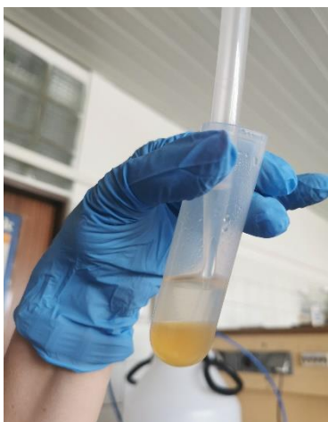
Fig. 4 Pre-extraction into ethyl acetate (3 times by 5 mL of ethyl acetate; collection of the upper layers into evaporation flask)
