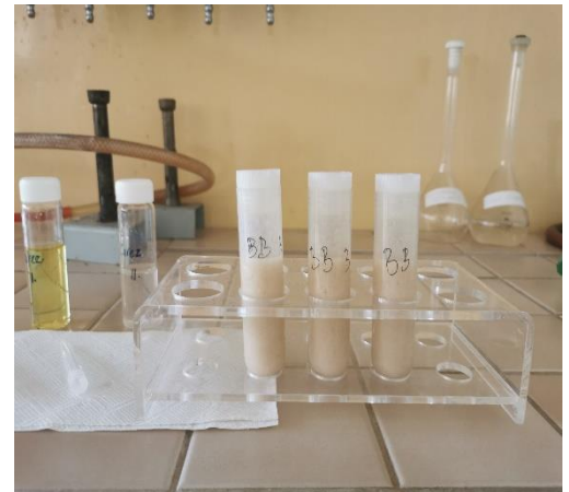
Fig. 2 Acrylamide water extraction by 0.1 % of acetic acid and clarification by Carrez solutions
